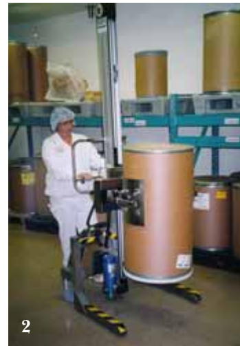
2. PRO200 with EasySqueeze unit, stainless steel.
