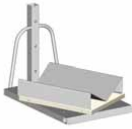
152A/B/C/D Adjustable forks for PRO120/150 frame 102A. A: 80 kg 40x20 mm l: 500 mm. B: 60 kg 30x30 mm l: 500 mm. C: 40 kg 20x20 mm l: 400 mm D: 40 kg dia 25 mm l: 450 mm. Reaches floor level.
