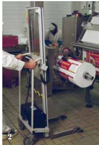
2. A PRO100 with EasySqueeze unit and electric turning. The arms hold and turn the roll, moving it from a vertical position to the horizontal, loading position.
