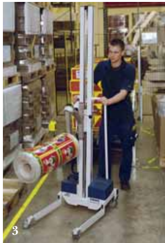
3-4. A coregripper tool grips the inside of the roll and rotates 90° from a vertical position to a horizontal position. PRO70 (left) PRO120 (right).
