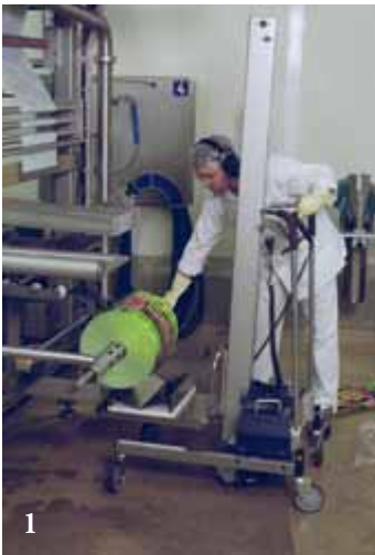
1. The PRO120 with V-block and rotating plate.
