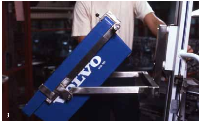
3. A manual crateturning tool, PRO70.
