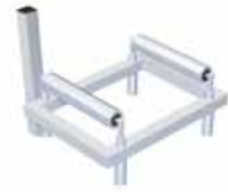
Special tool for handling tyres.
