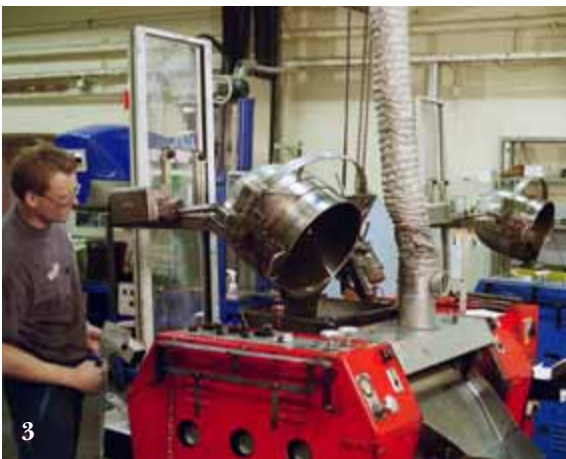
3. PRO100's with electrical turning tool.
