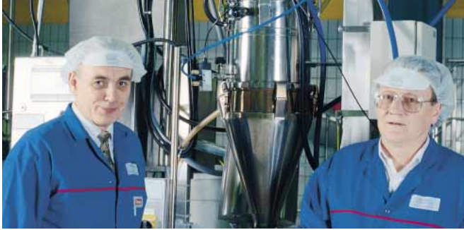
Karl-Axel Rydén and Kenneth Lindkvist at Nestlé with PIAB's vacuum conveyors, which contributed to a more hygienic handling of powdered mixes.
